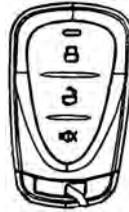
Smart key(remove the key after pressing the switch)
